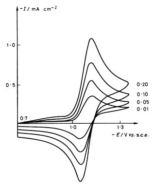
Figure 1. Cyclic voltammograms run between  $-0.6 \, \text{V}$  and  $-1.4 \, \text{V}$  for  $4\text{-NO}_2\text{C}_6\text{H}_4\text{CH}_2\text{OCONHC}_4\text{H}_9$  (1a) (2.5 mmol dm<sup>-3</sup>) in DMF-Bu<sub>4</sub>-NBF<sub>4</sub> (0.1 mol dm<sup>-3</sup>). Vitreous carbon disc electrode. Potential scan rates in V s<sup>-1</sup> as shown on the Figure
