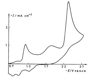
Figure 2. Cyclic voltammogram of 4-NO<sub>2</sub>C<sub>6</sub>H<sub>4</sub>CH<sub>2</sub>OCONHC<sub>4</sub>H<sub>9</sub> (1a) over a wide potential range at a scan rate of 0.2 V s<sup>-1</sup>. Other conditions as Figure 1
