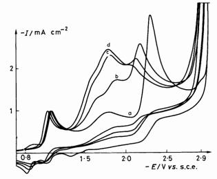
Figure 3. Cyclic voltammograms of  $4\text{-NO}_2\text{C}_4\text{H}_4\text{CH}_2\text{OCON-c-}(\text{CH}_2)_5$  (1d) (2.5 mmol dm<sup>-3</sup>) in DMF-Bu<sub>4</sub>NBF<sub>4</sub> (0.1 mol dm<sup>-3</sup>) containing methanol (a) 0%; (b) 2%; (c) 5%; (d) 8%. Vitreous carbon disc electrode. Potential scan rate 0.1 V s<sup>-1</sup>
